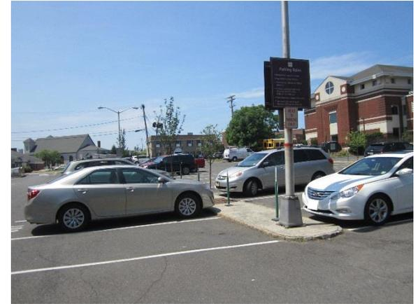
Parking spaces can be replaced with pervious pavement to capture and infiltrate stormwater. Installing bioretention systems adjacent to the building can capture, treat, and infiltrate roof runoff. A preliminary soil assessment suggests that more soil testing would be required before determining the soil's suitability for green infrastructure.
