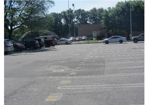
Parking spots can be replaced with pervious pavement to capture and infiltrate stormwater. Rain gardens can be installed to capture, treat, and infiltrate roof runoff. A preliminary soil assessment suggests that more soil testing would be required before determining the soil's suitability for green infrastructure.
